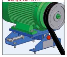
Generally retensioning is not necessary, however, we recommend to inspect the belt tension after a few days of operation.
