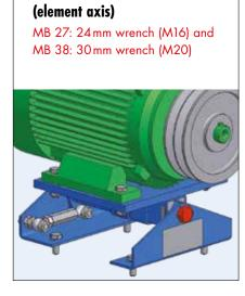
4 Loosen of the shaft bolt
