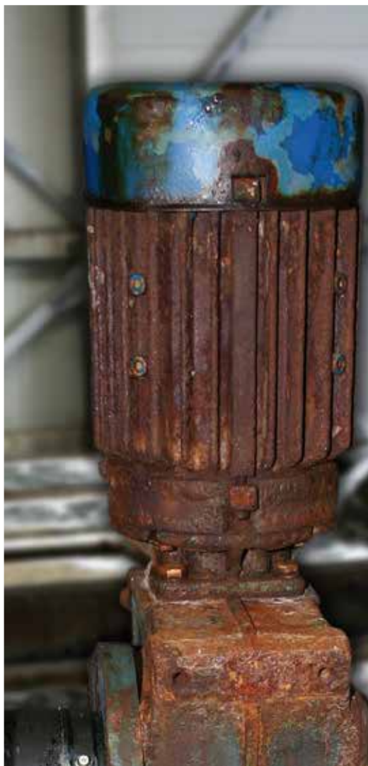
Painted gear motor after 12 months of use
