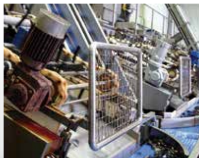
Painted gear motor after 12 months of use
