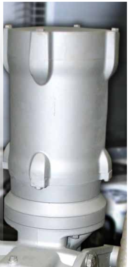
nsd tupH treated gear motor after 12 months of use
