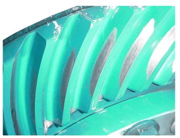
Load-bearing pattern made visible on a bevel gear.
